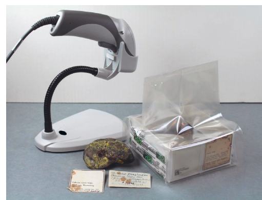
Figure 1. A pyritic ammonite, acid-burned labels, a completed anoxic microenvironment (with barcode inside) and a handheld barcode scanner.
