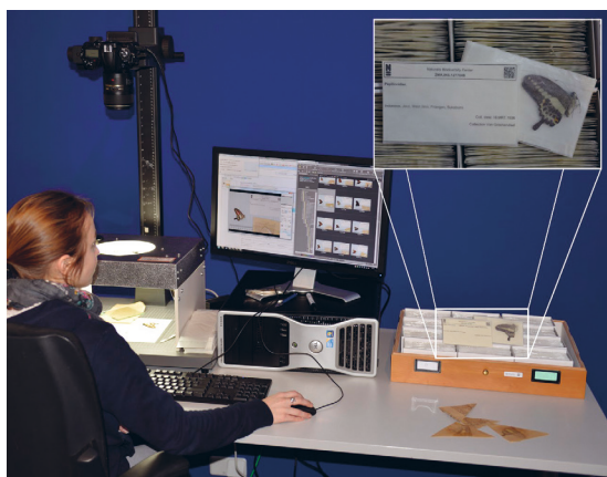
Figure 1. The handling step of the proposed workflow. It shows the original paper folds, the camera setup, the computer showing the camera's Live View and the permanent storage of unmounted Lepidoptera in glassine envelopes.
